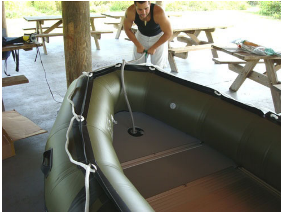
Last step is to inflate keel of the boat with a hand pump.
