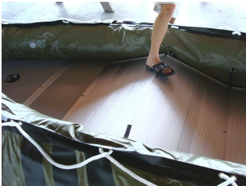
Step on raised part of two connected floor sections.
