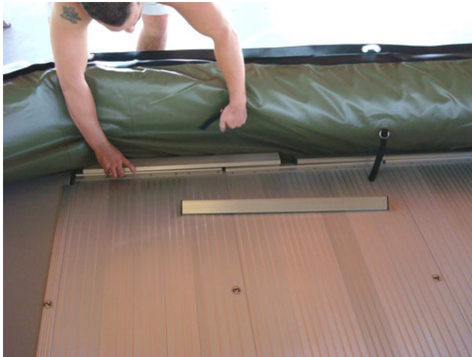
Aluminum stringers should interconnect at least two sections of the floor.
