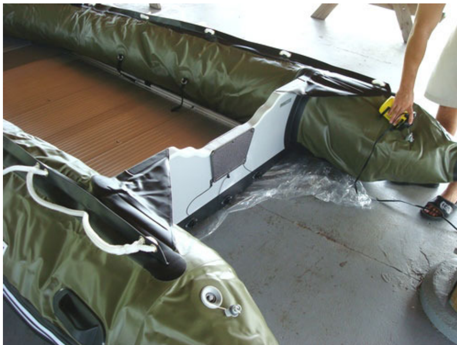
Inflate left and right tube of the boat. Use hand pump to finish.
